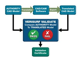
pass/fail result, and generates a complete report that will satisfy auditors the requirement has been met. Verisurf Validate can compare any two file types before and after import (translation) into Verisurf. The optional Validate solution is completely integrated into Verisurf and is easily accessed directly from the main menu.
