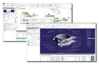
Simply drag a box around any dimension or MBD feature frame to enter callouts into the nominal column of a report. InspectionXpert uses character recognition to expedite data entry—reducing the frequent errors caused by traditional, manual entry methods. InspectionXpert is fully compatible with all Verisurf software configurations.
