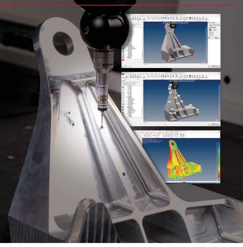
Verisurf Model-Based Inspection Software
